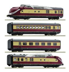
4-piece gas turbine multiple unit class 602 of the German Federal Railway.
