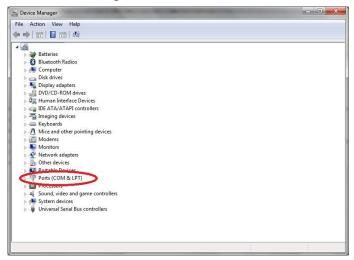
Check on which serial port is configured the Silicon Labs CP210x. In the example below it is configured on port COM4. The serial port must be specified when configuring the tOm Programmer.
