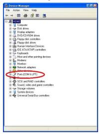
Check on which serial port is configured the Silicon Labs CP210x. In the example below it is configured on port COM8. The serial port must be specified when configuring the tOm Programmer.
