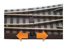
To program the decoder, it has to be passed into programming mode by manual switching the turnout five times between straight and branch position.
