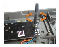
Mount the decoder to turnout carefully with the supplied screw in the decoders package.
