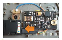
Between the 3-pin power connector of the decoder and the 5-pin one must remain one free pin at the actuator's connector.
