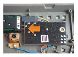
Insert the decoder in the electromagnetic actuator fitting the 5-pin connector in the drive's connector.
